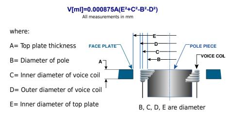
The recommended tolerance on ferrofluid quantity is  $\pm 10\%$  which is best maintained through the use of a positive volume displacement dispenser. Maintaining the proper ferrofluid quantity is critical as overfilling the gap is wasteful and can lead to leakage while underfilling the gap minimizes the heat transfer benefits of the ferrofluid, compromises the fluid's long term reliability and can lead to response anomalies in the loudspeaker.
