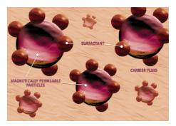
ferrofluid. In the absence of a magnetic field, the magnetic moments of the particles are randomly distributed and the fluid has no net magnetization.
